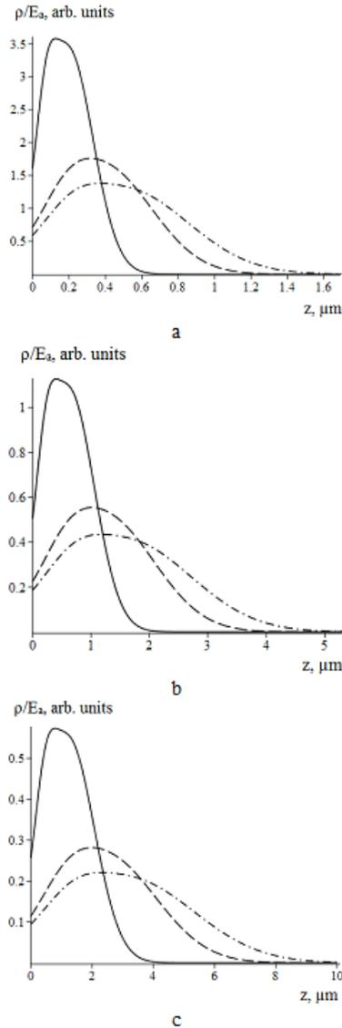
Fig. 1. Normalized to the power  $E_a$ , released in targets by an electron beam, energy losses by electrons in single-crystal gallium nitride (solid curves), silicon carbide (dashed lines) and silicon (dash-dotted lines). Energies of the beam electrons: 10 (a), 20 (b) and 30 (c) keV.
